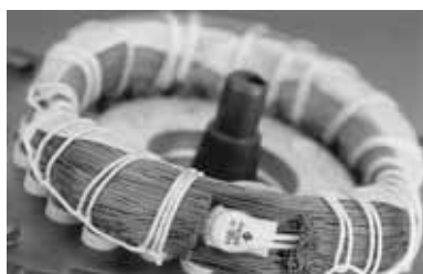
Fig. 28 Thermal switch incorporated in winding
