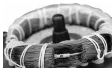
Fig. 26 PTC sensor incorporated in winding
